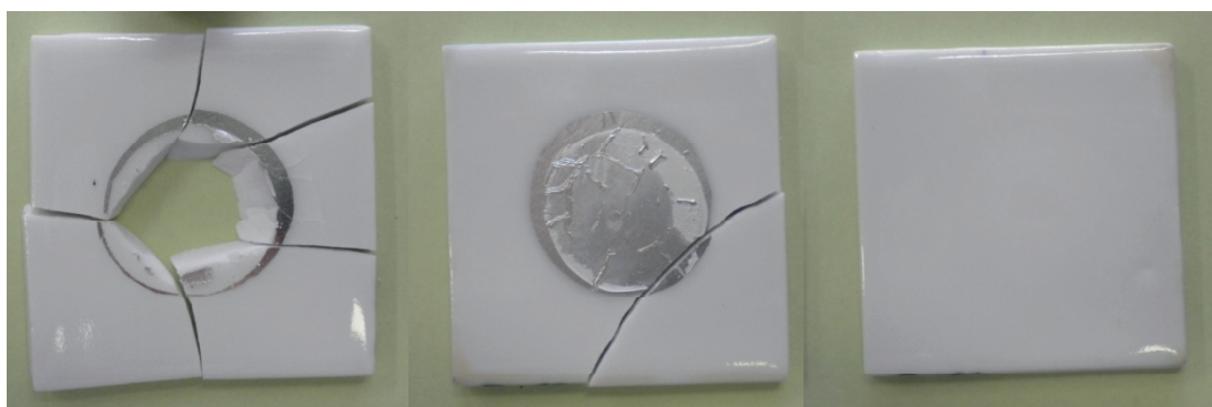
(a)母材破壊 (Al箔:5 \mu\text{m} )
