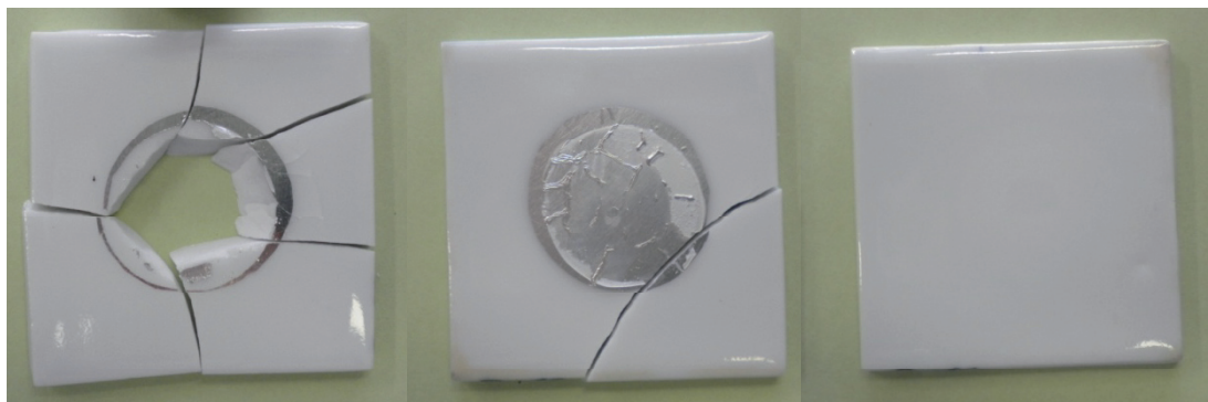
(a)母材破壊 (Al箔:5 \mu\text{m} )
