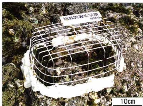
Fig.17 A net cage covering on S. fusiforme bed to protect from fish feeding. The cage was made of stainless steel wire and measured 35cm long × 30 cm wide × 18 cm high, with 5 × 4.5 cm mesh length.
